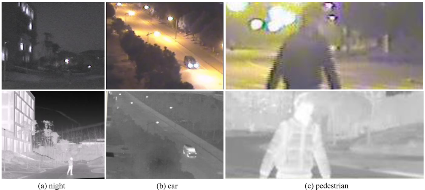
Fig. 1. Illustration of the heterogeneous foregrounds with different sizes in different modalities. The first and the second rows indicate the visible and thermal image pairs from GTFD dataset.
