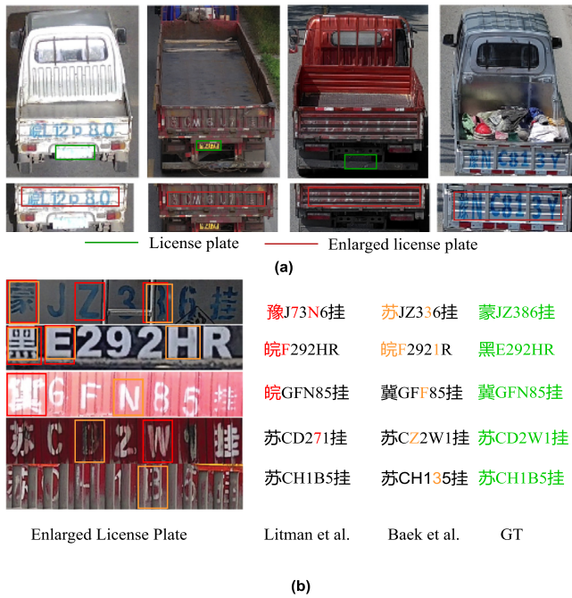
Fig. 1. (a) Comparison of enlarged license plates with standard license plates. Enlarged license plates are more suitable than standard license plates in identifying large vehicles under some challenging scenarios. (b) Recognition results of the enlarged license plates by the state-of-the-art recognition methods, including Litman et al. (2020) and Baek et al. (2019). All recognition models are trained using our proposed enlarged license plate dataset. The results show that the task of enlarged license plate recognition is challenging.
