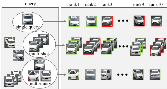
Fig. 1. Examples of ranking results comparison among the conventional single query, multi-shot and the proposed multi-query ReID on our collected MuRI dataset via ResNet-50 [15], where multi-shot (or multi-query) ReID is achieved by averaging the consecutive (or the different viewpoints) vehicle image features. The true and false matchings are bounded in green and red boxes, respectively.
